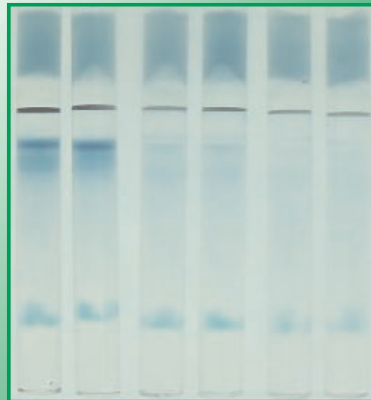
Figure 2. HDL Lipoprint® Gel Tubes after Electrophoresis of a Normal, Intermediate & Abnormal Human Serum Sample.
