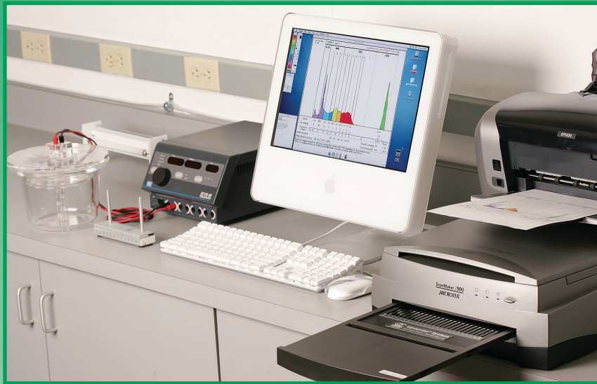
The Lipoprint HDL System consists of the reagent kit, preparation rack, preparation light, electrophoresis chamber, power supply, scanner and computer .
